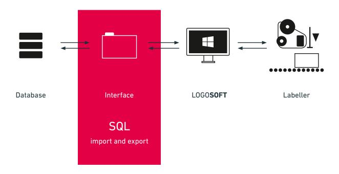
After the SQL interface has been set up, you need to create a source table (SQL Table or View) in your IT system for the data export. This source table contains all data required for the labelling process. The data is then automatically transmitted to your labeller via SQL.
